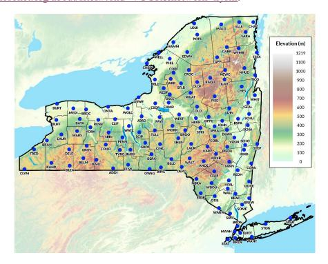
Each of the Mesonet's 126 weather stations collects observations of surface temperature, relative humidity, wind speed and direction, precipitation, solar radiation, atmospheric pressure, snow depth, and soil moisture and temperature at three depths (5, 25, and 50 cm). Each site is also outfitted with a camera that collects still images.
