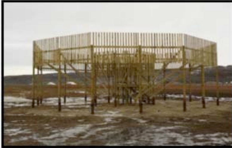
Figure 12: Double fence enclosure for the Geonor Snow Measurements at the Iqaluit Environment Canada Weather Office (photo by Gabrielle Gascon).
