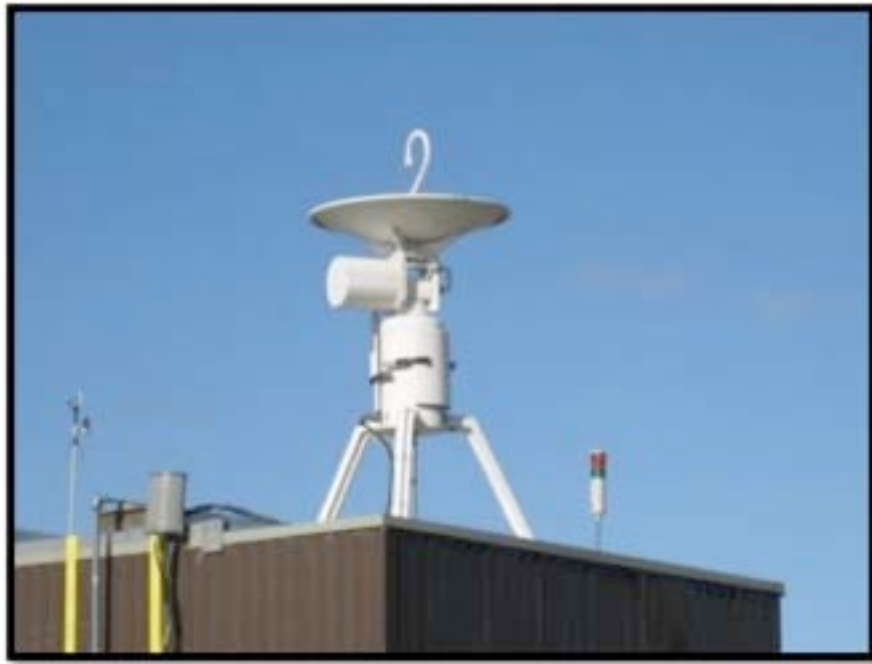
Figure 6: Portable X-band surface Doppler Radar at YFB Environment Canada Weather Office (photo by Robyn Dyck)
