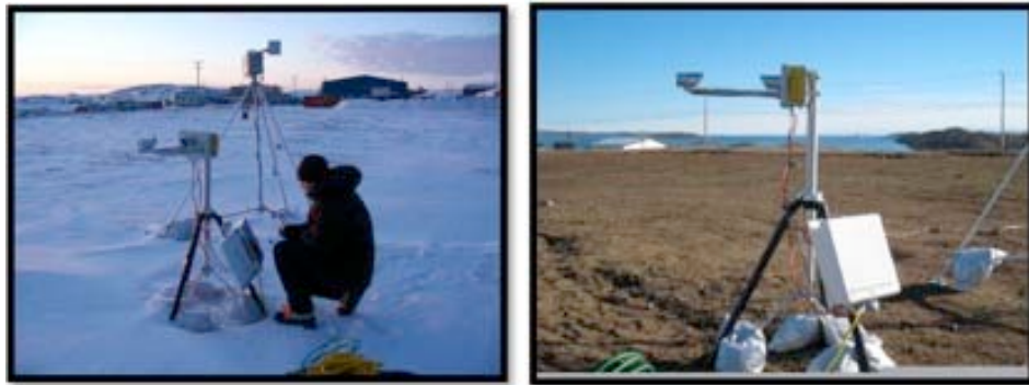
Figure 13: Laser Precipitation Sensor at YFB Environment Canada Weather Office (photos by Shunli Zhang (l) and John Hanesiak (r))
