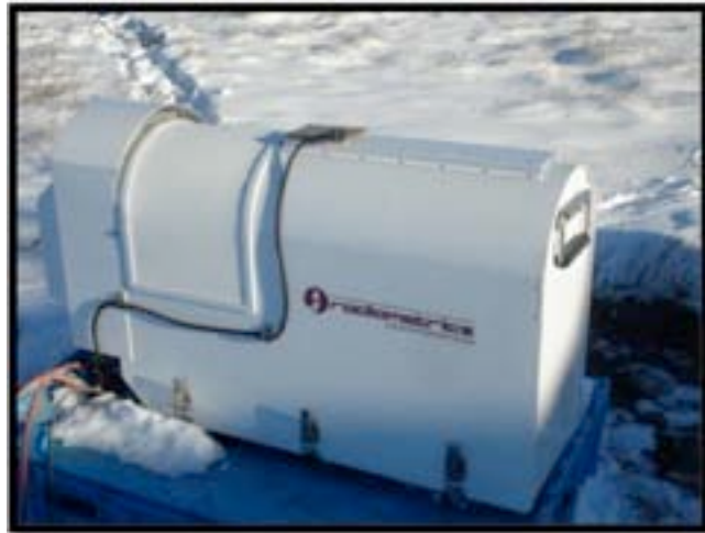
Figure 7: Microwave Radiometer at YFB Environment Canada Weather Office (photo by Robyn Dyck)
