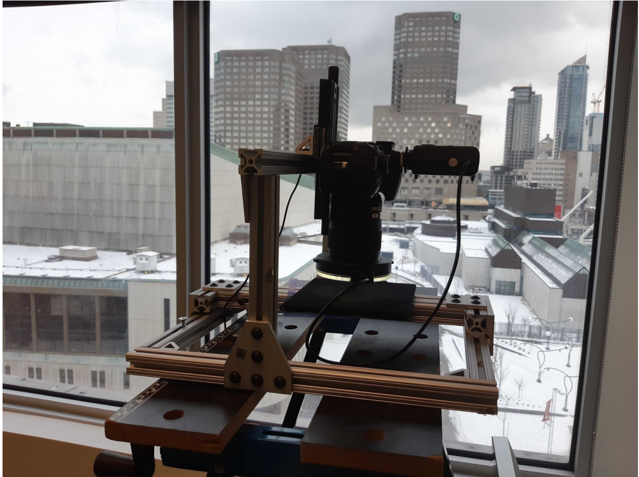
Figure 2.1 The metal base and the DSLR camera installed as they are used during precipitation events (adapted from Lachapelle & Thériault, 2022).
