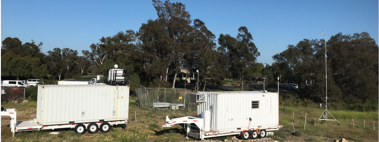
Figure 2. ISS instrumentation set up at the SBHQ site during SWEX. The Windcube lidar (sitting atop the trailer at left), the 449 MHz Modular Wind Profiler (in the center fenced area), and instrumented surface meteorology tower to the right can all be seen.
