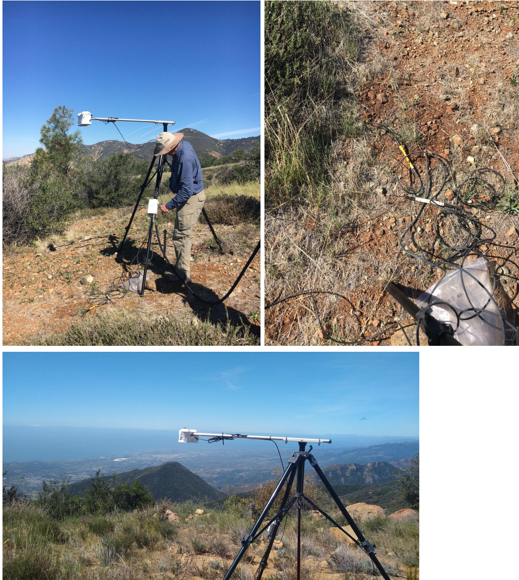
Photo 2. Radiometer set-up on tripod with soils buried at its base shown for s15 (Figueroa Mountain) - Top and s10 (La Cumbre).
