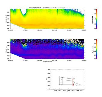
The aerosol layer in Figure 1 indicated by high backscattering and depolarization ratio below 3.5 km is apparent. The aerosol layer shows stronger wave patterns as the Twin Otter flew northward.
