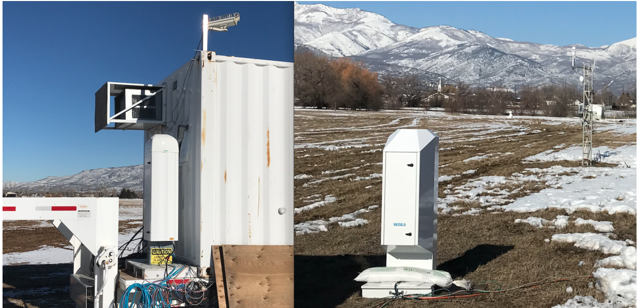
The ISS ceilometers at CFACT. The CL51 ceilometer was mounted on the front of the ISS1 trailer at the North Pivot site (left photo). The CL61 ceilometer was on the ground adjacent to the sounding trailer and met tower at the Deer Creek sounding site (right photo)..
