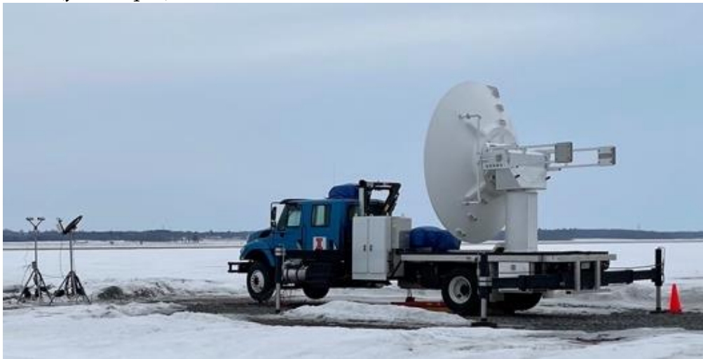
Fig. 2: Image of the MRR and disdrometer (left side) located at the COW radar site. Note that the instruments only ran when the COW was operating.
