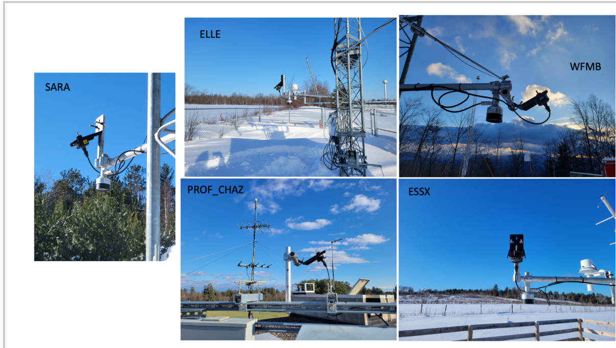
Figure 2: Photos showing the ice detectors mounted at each of the five stations. Photos are labeled with the station IDs given in Table 1.
