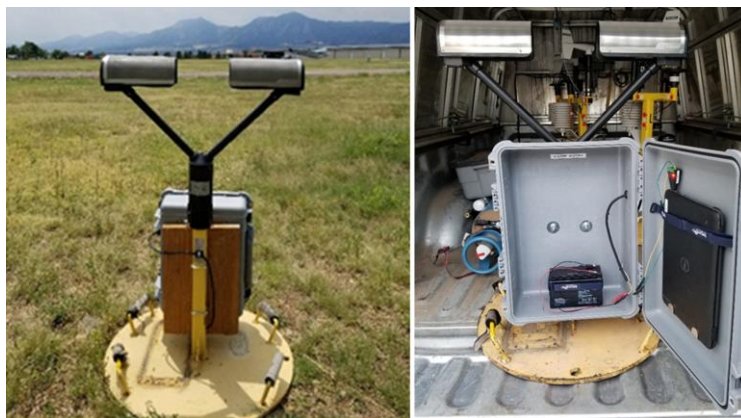
Figure 13: A FARM Parsivel2 disdrometer instrument deployed in a grass field (left) and on a SCOUT truck bed showing the battery and laptop installed within the Pelican case (right).
