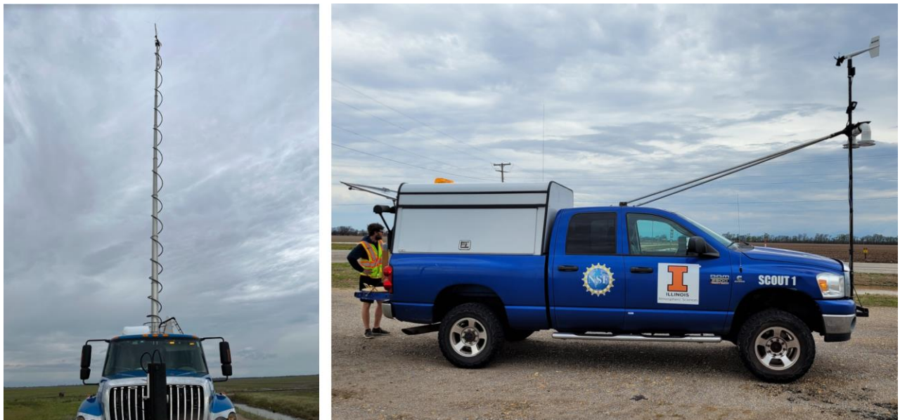
Figure 11: (left) DOW6 with its pneumatic mast fully extended and (right) SCOUT1 with its rigid mast. Mesonet instrumentation are mounted on the tops of each mast.
