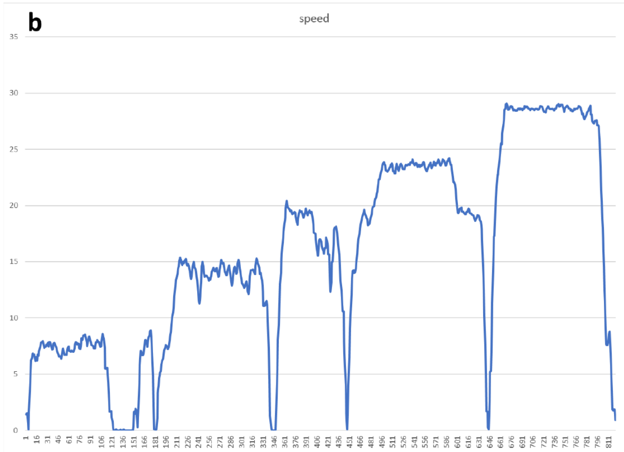
Figure 4: Calculated vehicle speeds from first segment of IOP 9 (Sedgwick Reserve to Buellton) in m/s. (a) Before correction for GPS lag effect; (b) after correction.
