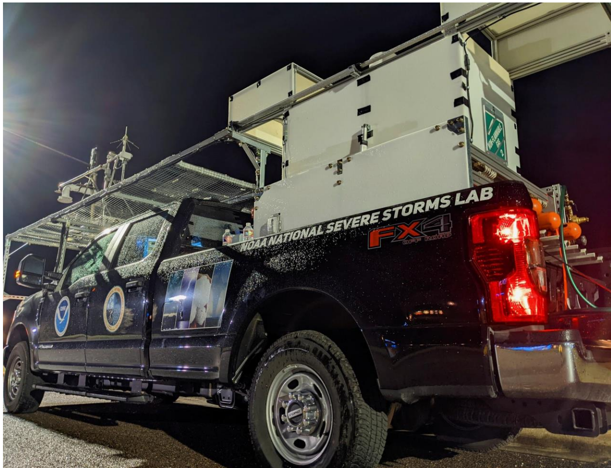
Figure 1. This photo shows the NSSL Doppler lidar truck as it appeared during PERiLS 2022 in deployment mode. The Doppler lidar's scanner head is visible protruding from the center of the open enclosure system in the back of the pickup truck. The truck also launched radiosondes and carried a mobile mesonet rack, which are separate datasets.
