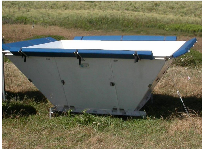
915 MHz phased array wind profiler
