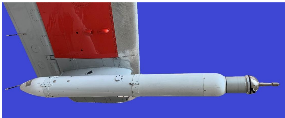
Figure 1. UHSAS-A (Port wing tip mounted UHSAS).
