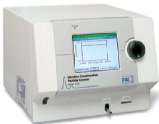
Figure 3. CPC 3775. Image by the manufacturer (TSI).
