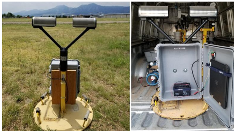
Figure 14: A FARM Parsivel2 disdrometer instrument deployed in a grass field (left) and on a SCOUT truck bed showing the battery and laptop installed within the Pelican case (right).
