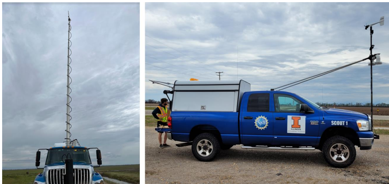
Figure 12: (left) DOW6 with its pneumatic mast fully extended and (right) SCOUT1 with its rigid mast. Anemometers and T/RH sensors are mounted at mast height.
