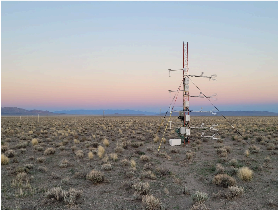
Photo 1B. View of t0 6m tower with Temperature, RH, P, h 2 O/CO 2 gas analysers, and 3D sonic sensors mounted at 0.5m, 1m, 2m, 3m, and 4m.
