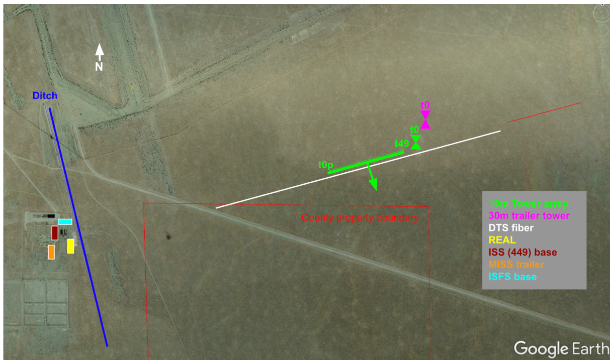
Schematic 1. Schematic rendering of horizontal array and 30m trailer tower, relative to the ISS and PI base operations.
