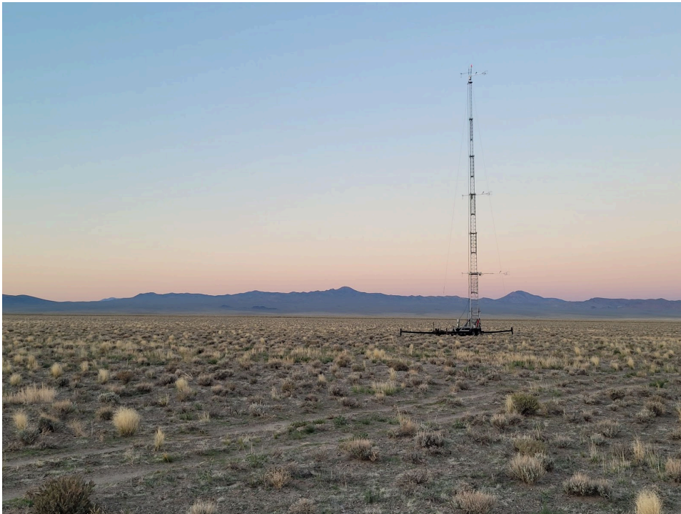
Photo 1C. View of t0 30m tower with Temperature, RH, P, h 2 O/CO 2 gas analysers, and 3D sonic sensors mounted at 7m, 15m, and 28m.
