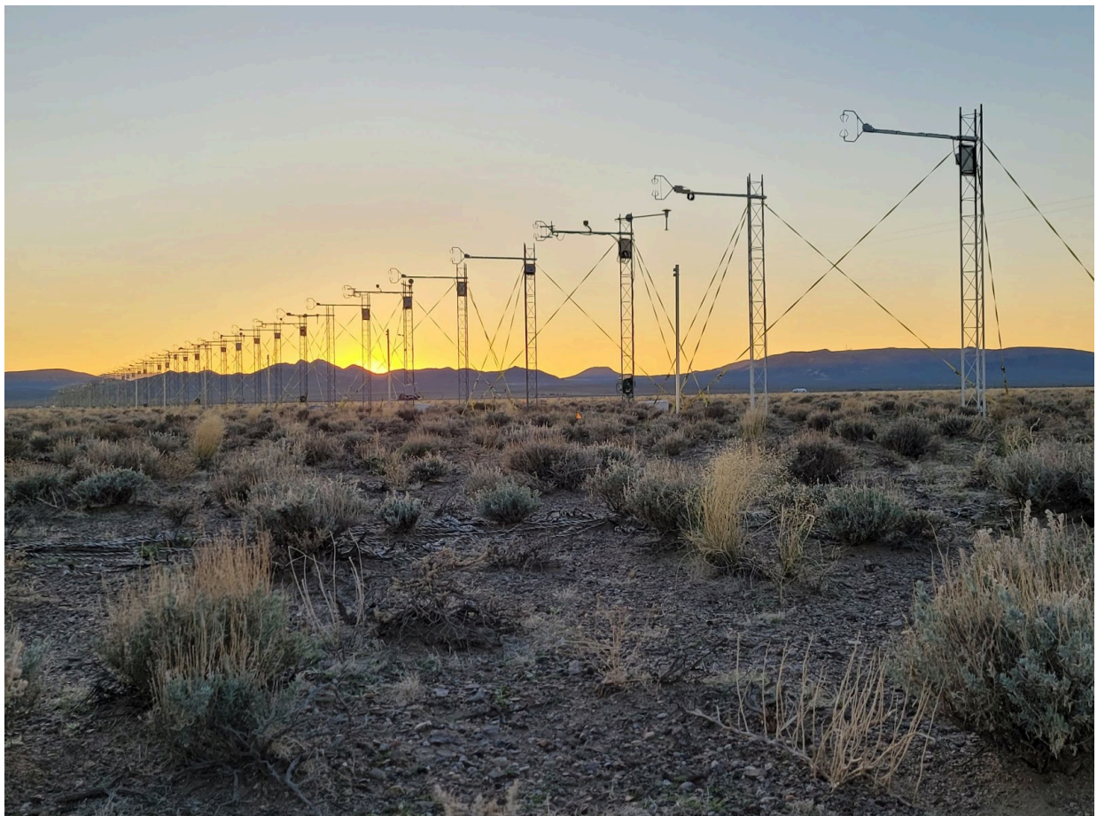
Photo 1A. View of a section of the horizontal array at sunset. 3D sonic anemometers are mounted facing towards the south.
