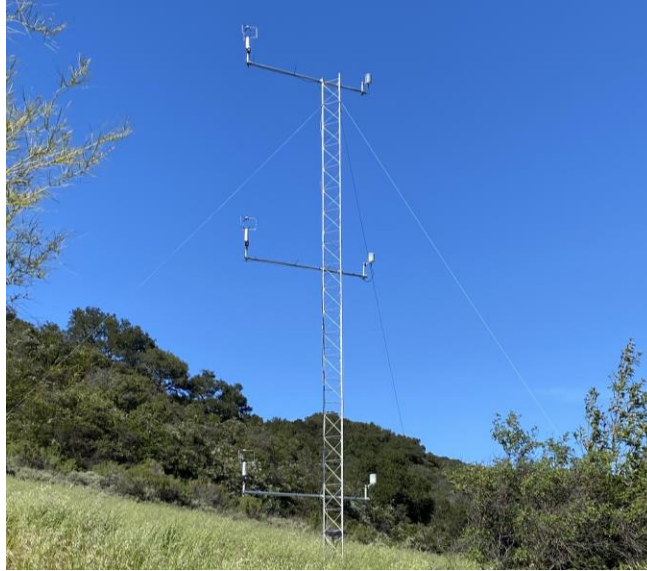
Photo 1: The location of the tower at HP. Sonic anemometers and temperature relative humidity probes are pictured at 2, 6, and 10 meters, along with a net radiometer at 2 meters above ground level.
