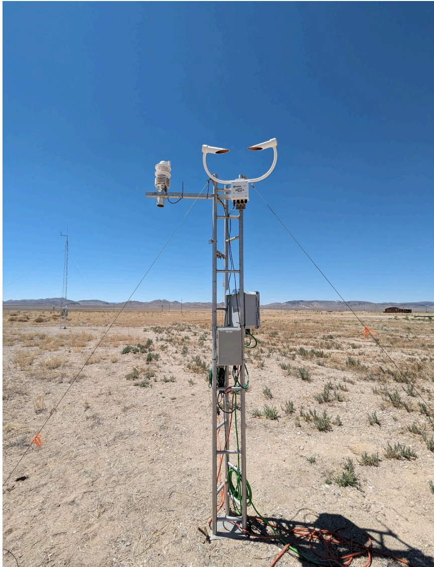
Photo 1. 3 m tower with the CS125 Visibility sensor and Lufft ws800 mounted at the top. The pressure, temperature, and RH from the Lufft ws800 was used as the surface reference sensor for the radiosondes. The 10 m tower is visible behind and to the left of this tower.
