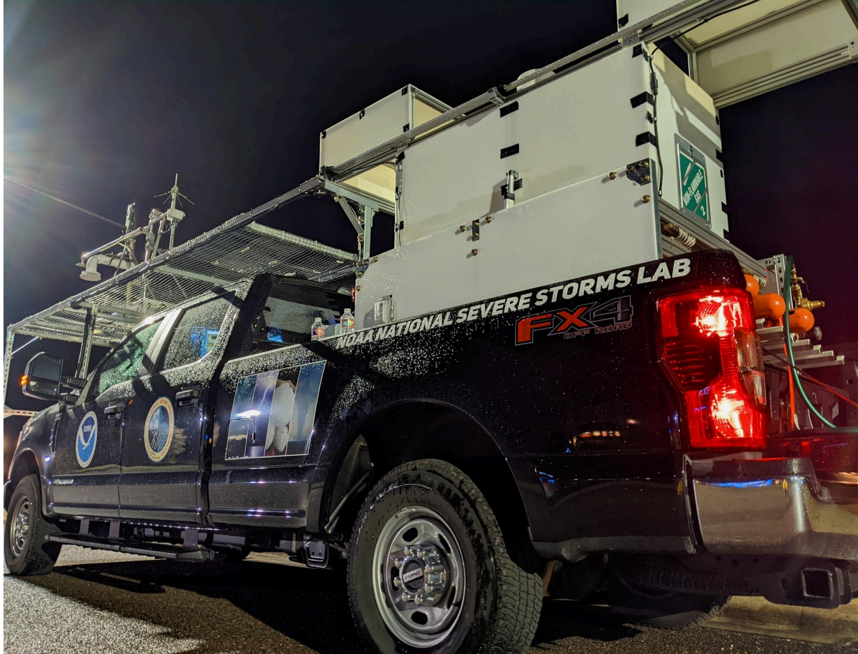
Figure 1. This photo shows the NSSL Doppler lidar truck as it appeared during PERiLS 2022 in deployment mode. This configuration is generally representative of the TORUS-Lite 2023 configuration. The Doppler lidar's scanner head is visible protruding from the center of the open enclosure system in the back of the pickup truck. The truck also launched radiosondes and carried a mobile mesonet rack, which are separate available datasets. The field catalog entries offer documentation of collocated radiosonde launches from the onboard system and occasional notes about Windsond launches from NSSL/CIWRO teams coordinating with our location.
