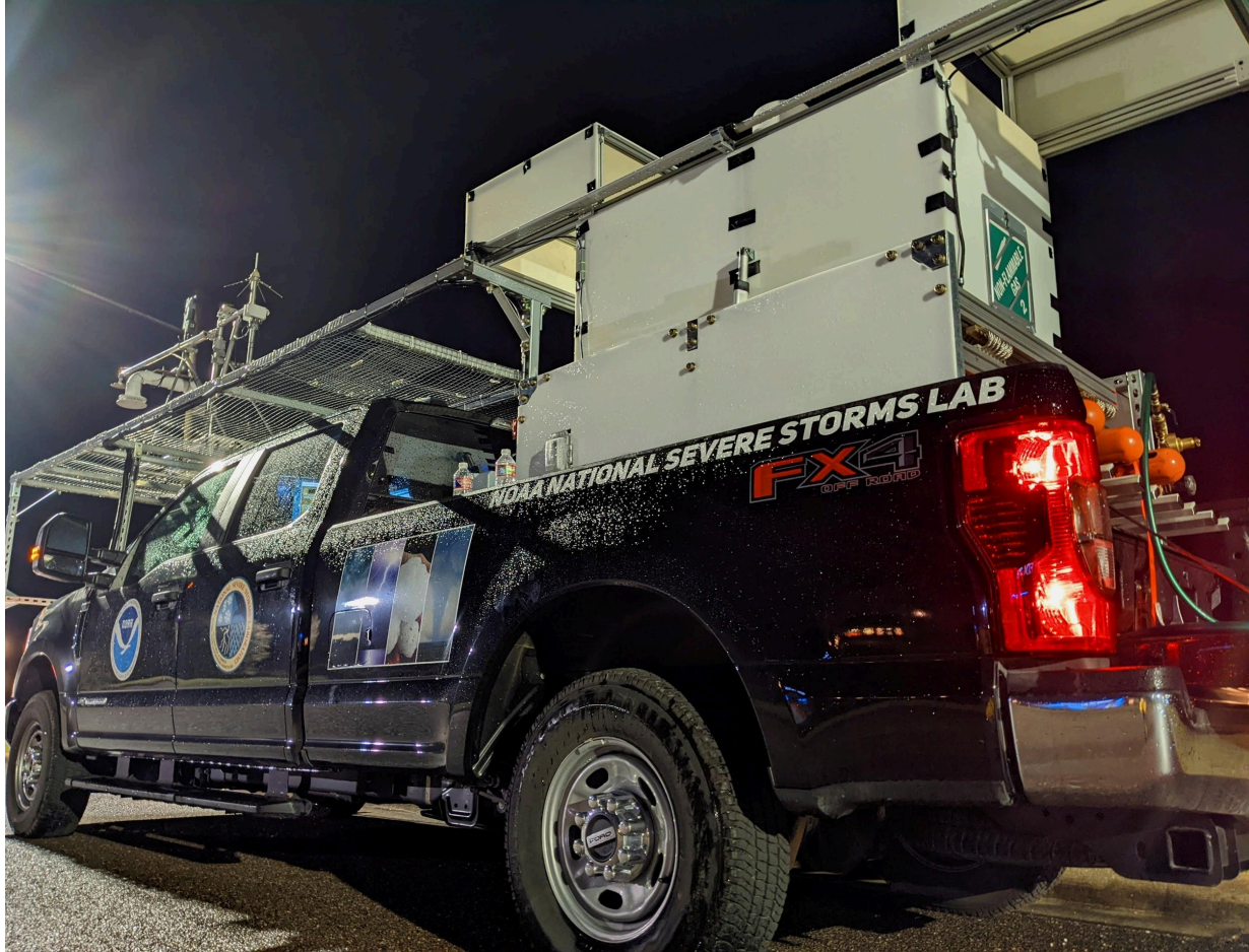
Figure 1. This photo shows the NSSL Doppler lidar truck as it appeared during PERiLS 2022 in deployment mode. This configuration is generally representative of the TORUS-Lite 2023 configuration. The Doppler lidar's scanner head is visible protruding from the center of the open enclosure system in the back of the pickup truck. The truck also launched radiosondes and carried a mobile mesonet rack, which are separate available datasets. The field catalog entries offer documentation of collocated radiosonde launches from the onboard system and occasional notes about Windsong launches from NSSL/CIWRO teams coordinating with our location.
