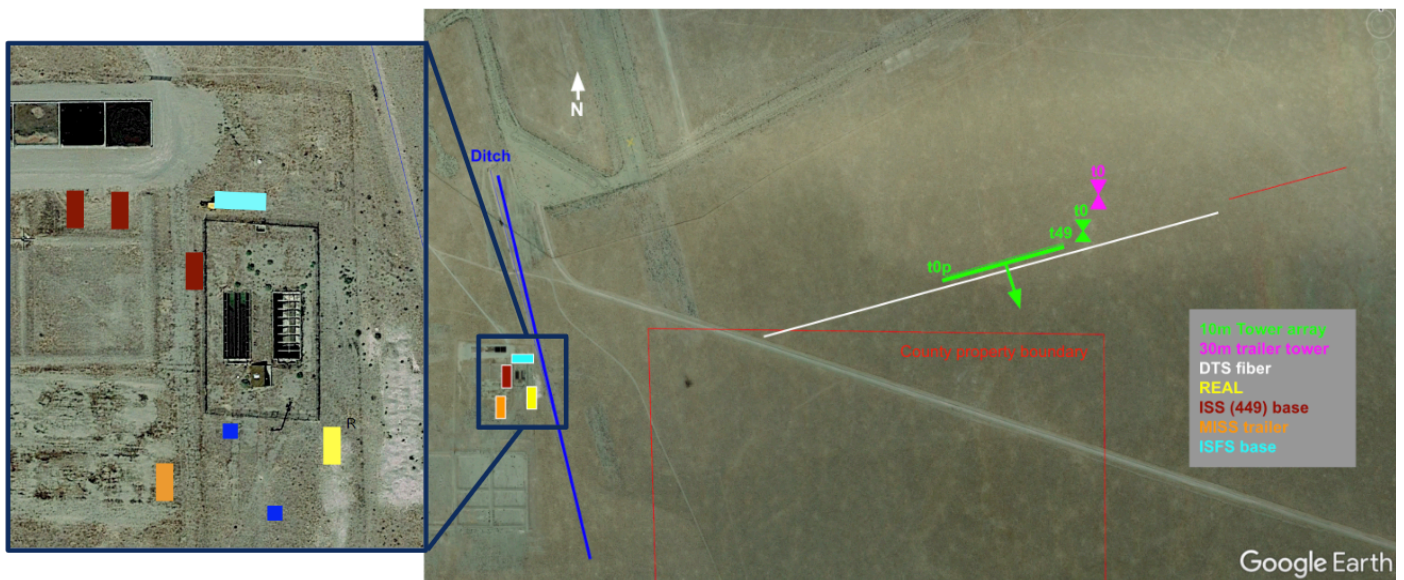
Schematic 1. Schematic of the overall set-up, in terms of ISS trailer and instrument suite location relative to the ISFS towered flux array.
