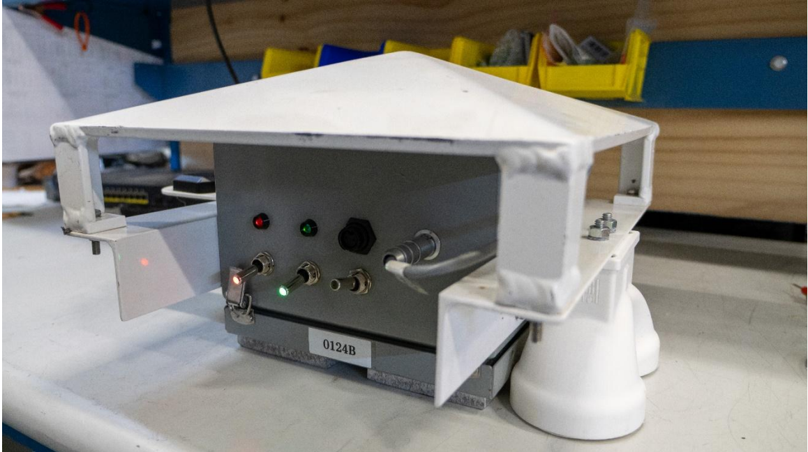
Figure 1. Photograph of the impact disdrometer impact plate and data acquisition enclosure assembly. Also note on the right side of the plate frame is the aspirated thermodynamic sensor package, which is a modified and scaled down U-tube style assembly.
