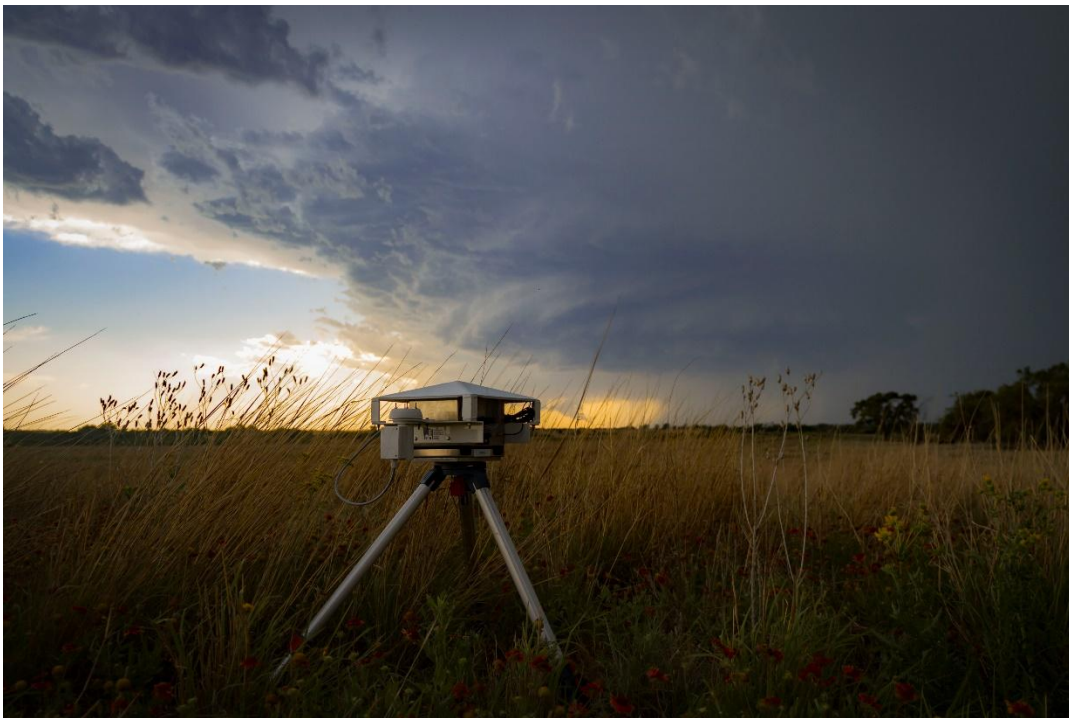
Figure 2. Photograph of an IBHS hail disdrometer deployed in the field in 2017.
