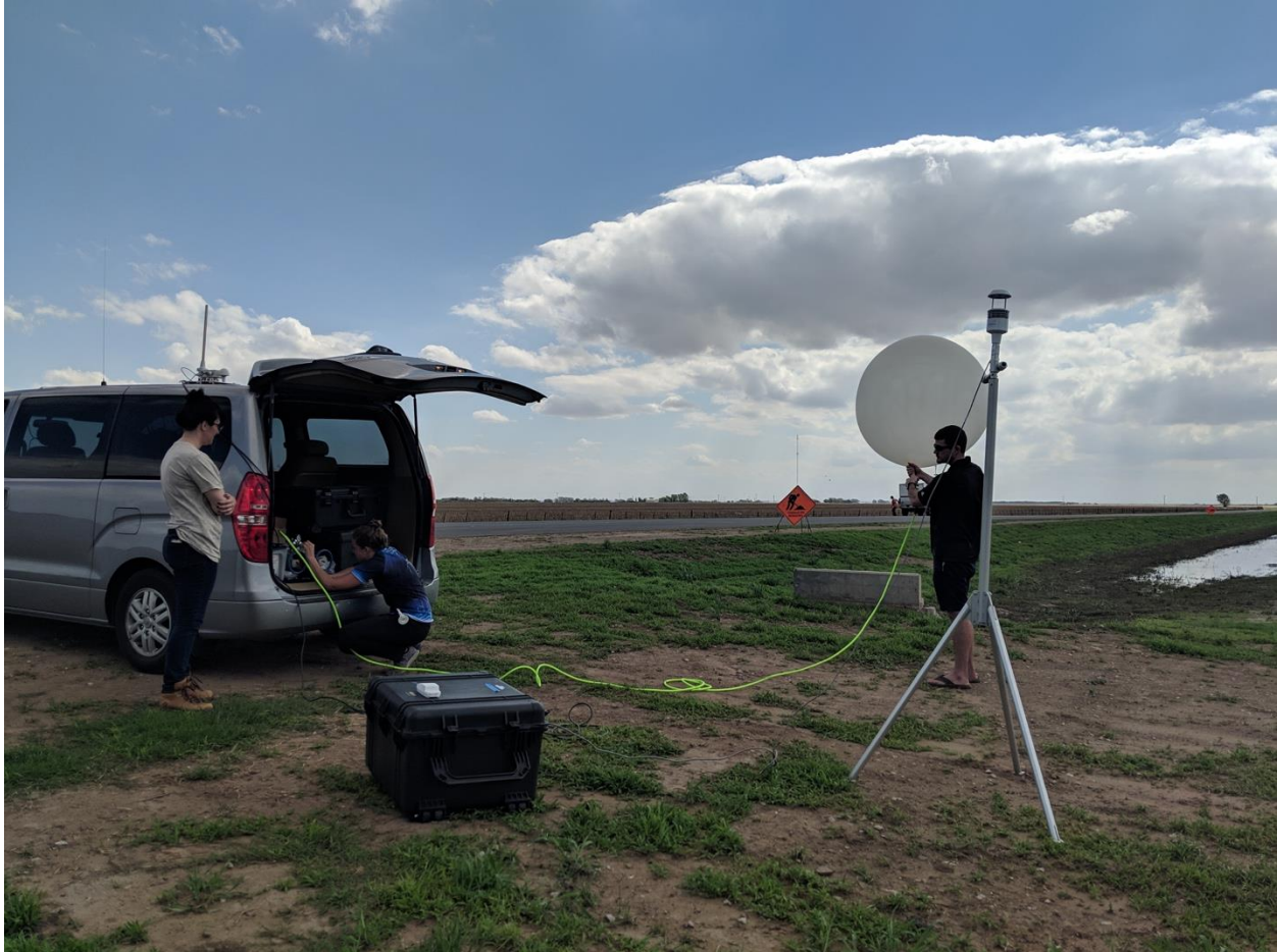
Figure 1: Photo showing typical setup of all-in-one surface station (foreground) with respect to vehicle during a CSU deployment.
